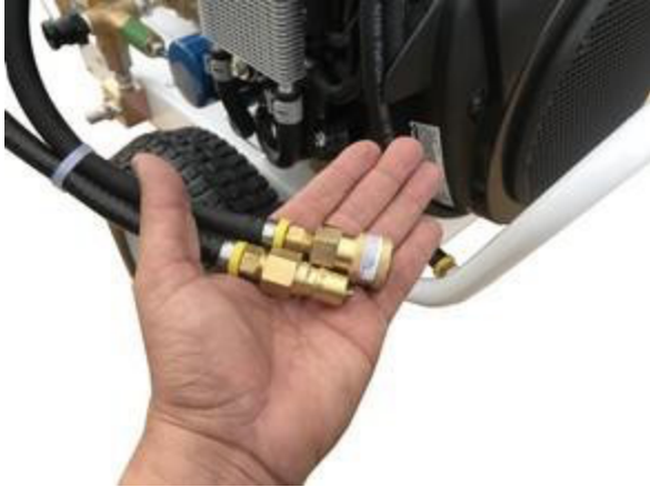
Figure #13 – Dual Fuel Lines
