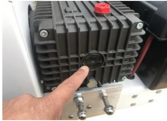
Figure #2 – Oil Level in Pressure Pump
