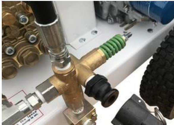
Figure #30 – Pressure Regulating Unloader
