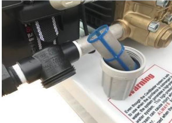
Figure #1 – Inlet Water Strainer
