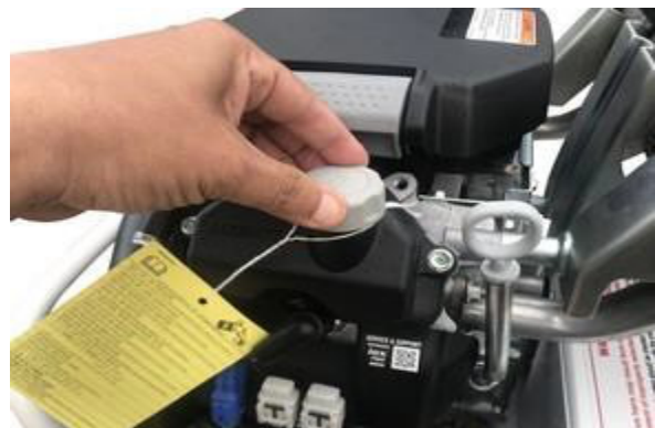
Figure #6 – Oil Filling Port in Engine
