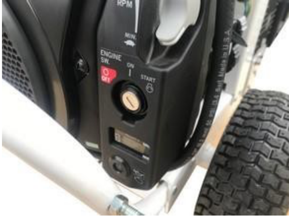
Figure #19 – Ignition Panel
