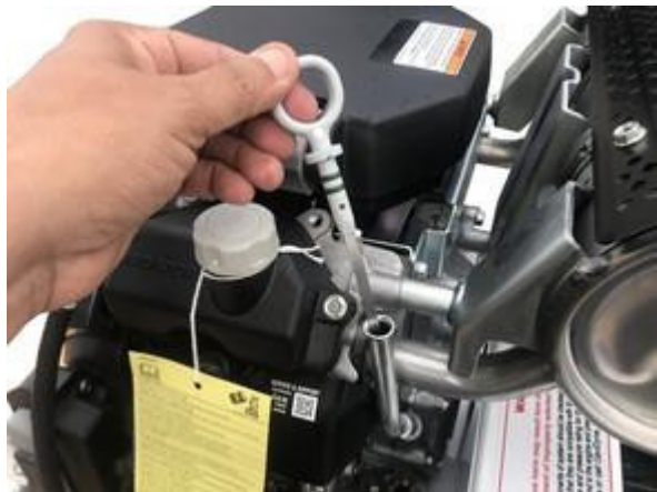
Figure #3 – Oil Level in Engine
